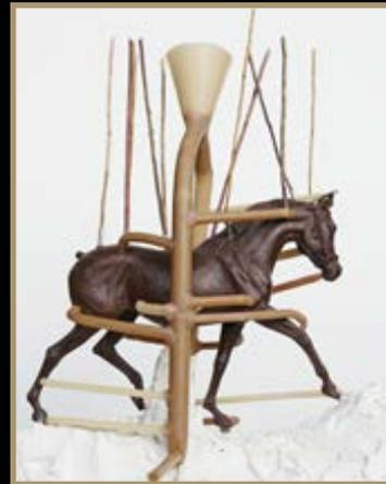
5. This complex system is necessary for leading melted hot bronze into the mold and at the same time the air out of it
